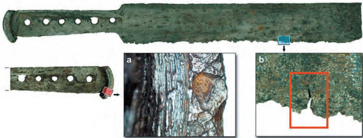
Fig. 14. Selected details of the dussack from Horákov: a – layering visible under the pommel; b – a quenching crack in the cutting edge of the dussack
